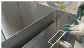
Put the lip seal on the edge all the way to the around and to the starting point
