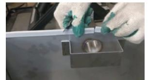
Remove excess silicone, put the cover back on firmly and close the quick-release fasteners
