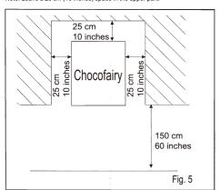
Fig. 5 shows the clearances required for access:
