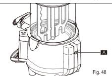
use a suitable tool to press the button inside to restore normal machine operation
