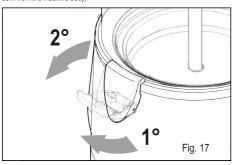
slide the mixing auger upwards with one hand, taking care to grip it by the rotation pin;
