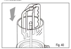
Fix the bowl to the machine body using the relevant hook-on handles, as illustrated in the figure;
