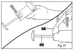
insert the mixer auger into its seating;
