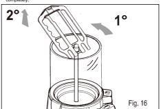
• unhook the bowl hook-on handles, as illustrated in the figure, to free the bowl from the machine body;
