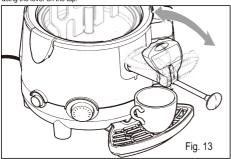
Fill the bowl with water and set the thermostat to 50°C (122°F). Operate the appliance for at least 15-20 minutes; increasing this amount of time will release any product residues that may be stuck to the sides of the bowl. Empty out the entire contents of the bowl, using the lever on the tap.
