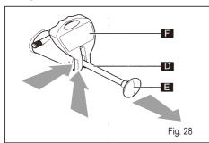
unscrew the knob (E) by turning it anticlockwise while holding the rod in place;
