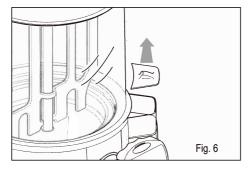
fill the boiler tank with water using the boiler tank level indicator tray, until it reaches the maximum value indicated on the tray itself, which is marked -MAX-:
