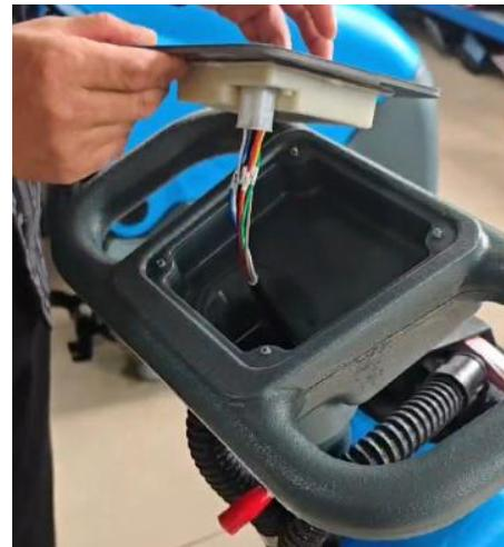
2. Use the corresponding tools (M6 screw driver) to turn the screw inside according to the picture on the right. Remember that you don't need to tighten the screw, but rotate it left and right until the handle is stable.
