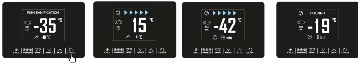
During a sanitation cycle, the device will always display the cabinet temperature and, depending on the phase in progress, the blast chilling end temperature or the duration of the holding phase.
