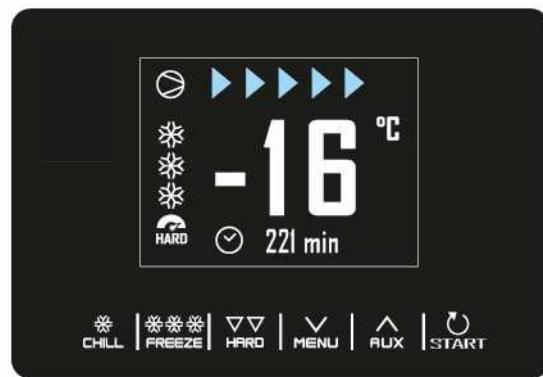
On completion of the blast chilling/blast freezing cycle, when the needle probe has reached the right temperature or the time period is finished, the buzzer sounds and the conservation phase begins. If the temperature controlled cycle is not completed in the allotted time, the problem will be notified by displaying an alarm message.
