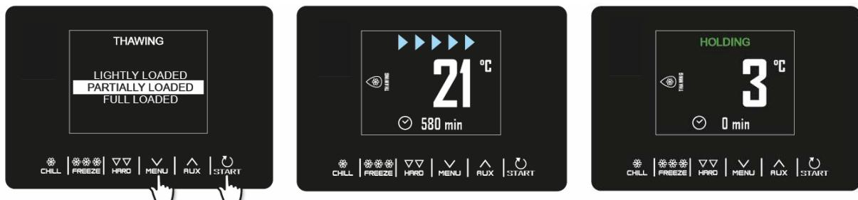
The defrosting cycle is managed on the basis of the amount of product to be defrosted that is loaded into the unit in relation to the maximum quantity specified by the manufacturer. To keep it simple, the load quantities that can be selected are divided into three bands, for each of which the controller will load three different sets of predefined parameters, in accordance with the following scheme:
