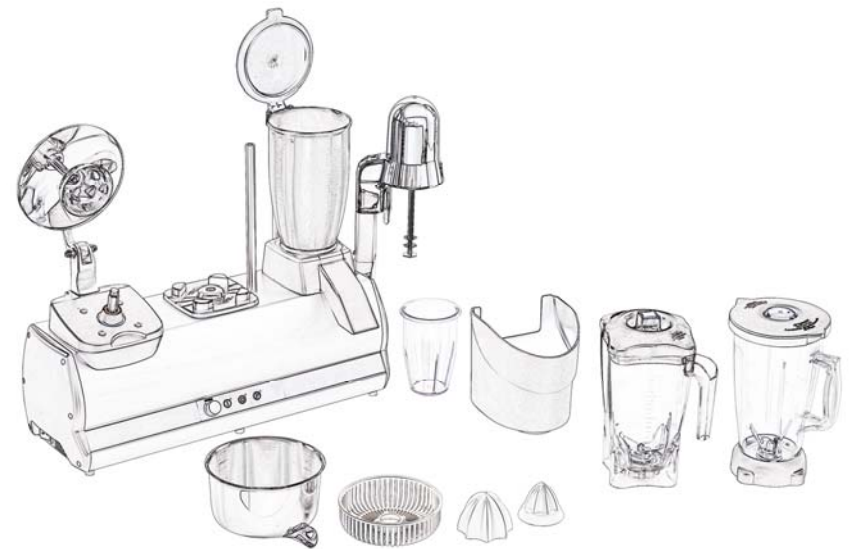
FIG. n°13 - Machine disassembled for the cleaning
